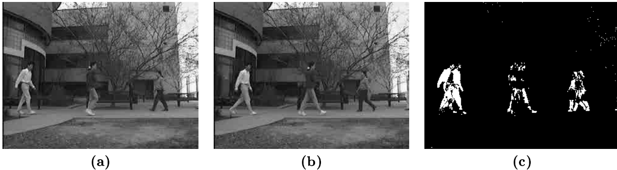
Figure 1: Images of the walkway near ENB at two time instants are shown in (a) and (b). Difference image, thresholded with a value of 40 gray levels, is shown in (c).
